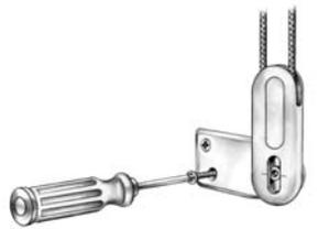
Pull the screw hole down and center it on the indicator line.
