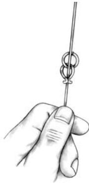
③ Push the lift cord between the open end of the breakaway ring until it moves freely inside the ring. Repeat for all rings that have broken away.
