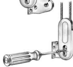
**Pull the screw hole down and center it on the indicator line.**
