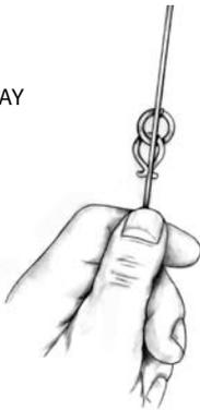
② Line up the lift cord with the open end of the breakaway ring.
